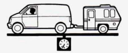
If your vehicle comes with the Trailering Package, there is also a load rating which includes the weight of the vehicle **and** the trailer it tows. This rating is called the Gross Combination Weight Rating (GCWR).
